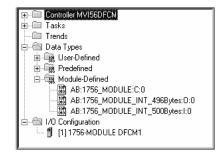
Next, define the User Defined Data Types to be used with the module. Copy these data types from the example ladder logic if you are not using the example. They will be defined if you are starting from the example ladder logic. The Controller Organization window should display the User Defined Data Types shown below:
