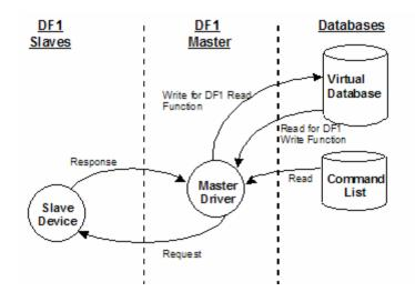
Each command issued from the DF1 master contains a field that indicates the location in the virtual database to be associated with the command. Care must be taken when designing a system to be sure the read and write data regions for the database do not overlap for a single device. The read area of one device can overlap the write section of another device to transfer the data from one slave device to another.
