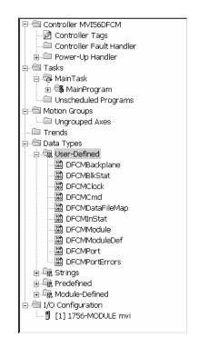
Next, define the data to be used to interface with the module and the ladder logic. Open the Controller Tags Edit Tags dialog box and enter the values shown in the following example. The MVI56-DFCM module is defined in the example as DFCM1. You can set the tag name to any valid tag name you desire. If you are using the example ladder logic, this step has already been performed.
