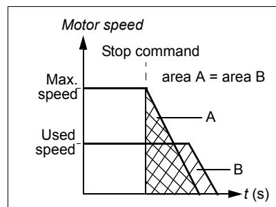
Speed compensation can be restricted to forward or reverse rotating direction.
