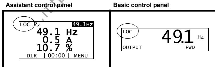
The control panel always overrides the external control signal sources when used in local control.
