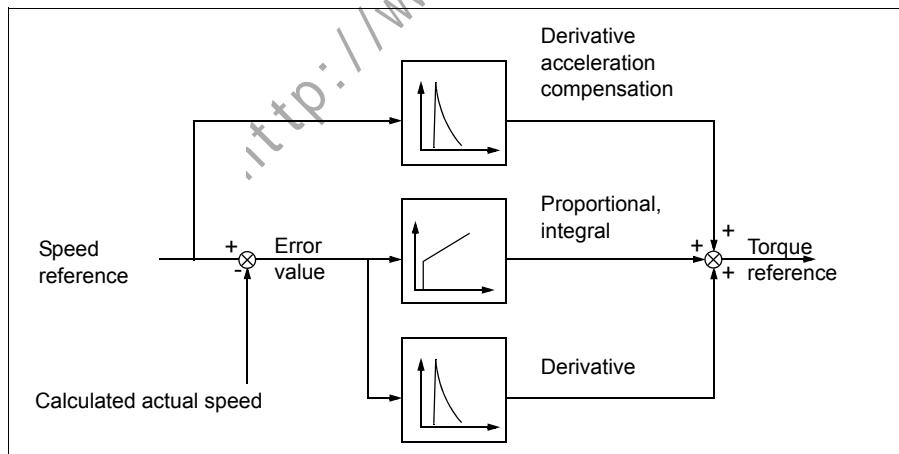
**Note:** The speed controller can be used in vector control, ie, when **9904 MOTOR CTRL MODE** setting is **VECTOR: SPEED** or **VECTOR: TORQ**.
