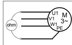
**Note:** Moisture inside the motor casing will reduce the insulation resistance. If moisture is suspected, dry the motor and repeat the measurement.
