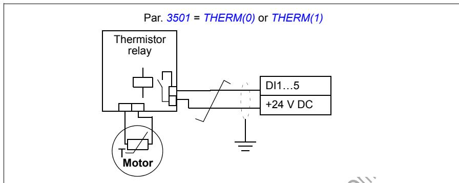
**WARNING!** According to IEC 60664, the connection of the motor thermistor to the digital input requires double or reinforced insulation between motor live parts and the thermistor. Reinforced insulation entails a clearance and creeping distance of 8 mm (0.3 in) (400/500 V AC equipment).
