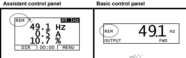
The user can connect the control signals to two external control locations, *EXT1* or *EXT2*. Depending on the user selection, either one is active at a time. This function operates on a 2 ms time level.
