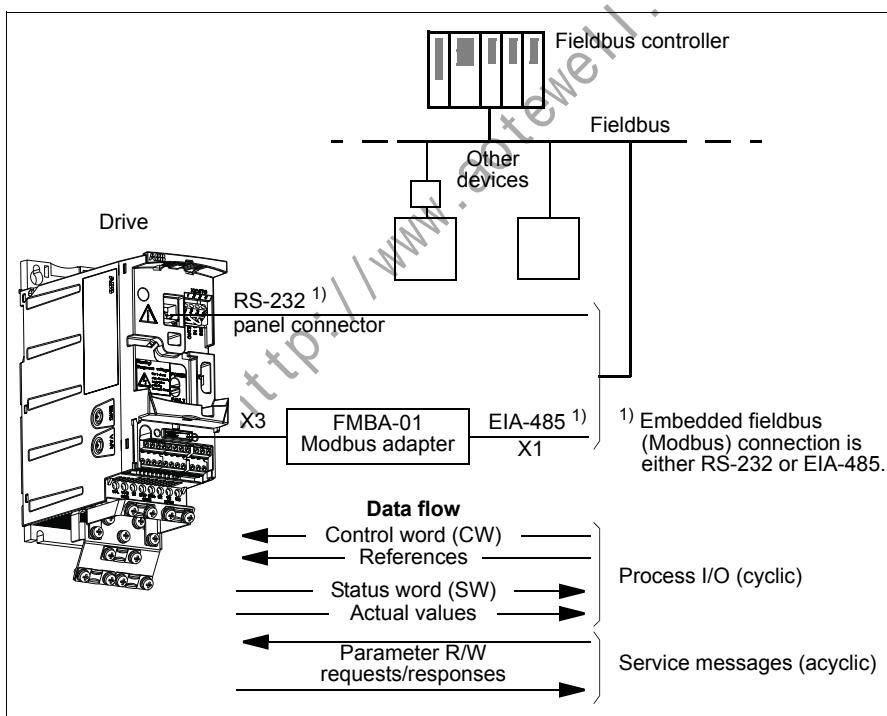
The drive can be set to receive all of its control information through the fieldbus interface, or the control can be distributed between the fieldbus interface and other available sources, for example, digital and analog inputs.
