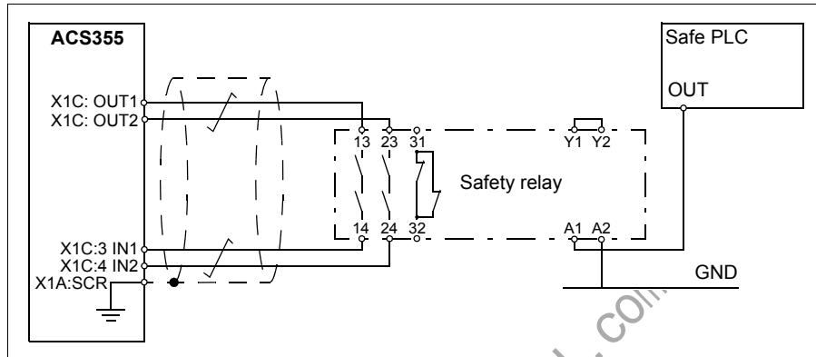
An example of a Safe torque off wiring with external +24 V DC power supply is shown below.
