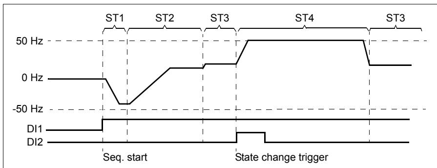
Sequence programming is activated by digital input DI1.
