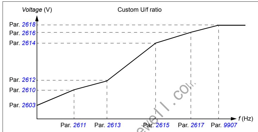
**Note:** The U/f curve can be used in scalar control only, ie, when **9904 MOTOR CTRL MODE** setting is **SCALAR: FREQ**.
