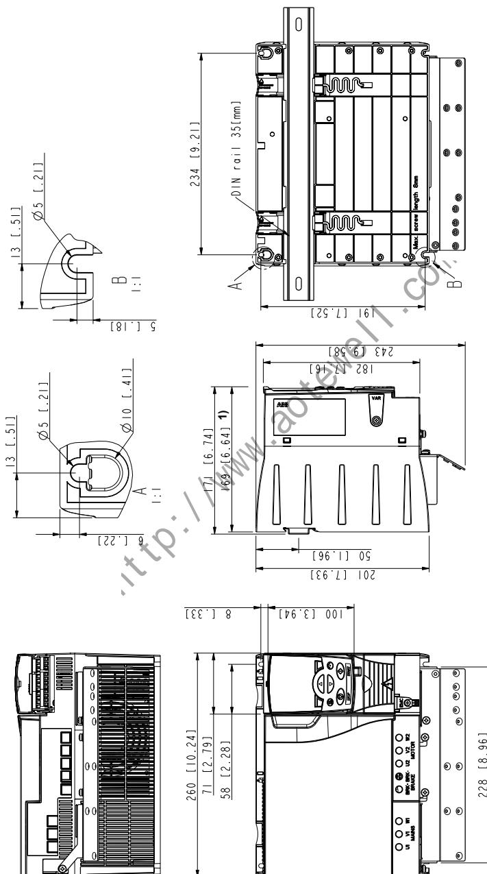
1) Extension modules add 26 mm (1.02 in) to the depth measure.
