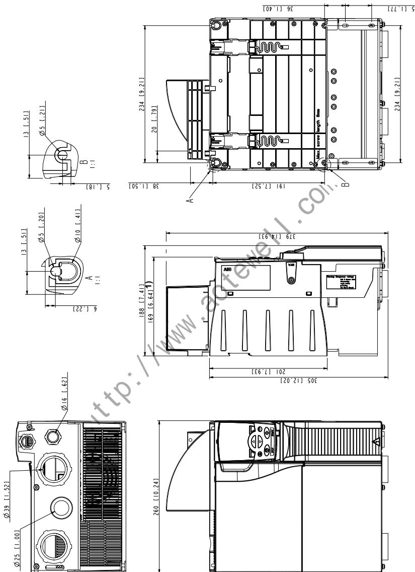
1) Extension modules add 26 mm (1.02 in) to the depth measure.
