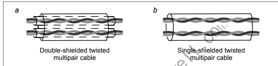
Run analog and digital signals in separate cables.
