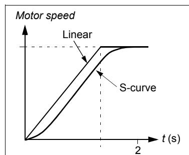
S-curve shape is ideal for conveyors carrying fragile loads, or other applications where a smooth transition is required when changing the speed.
