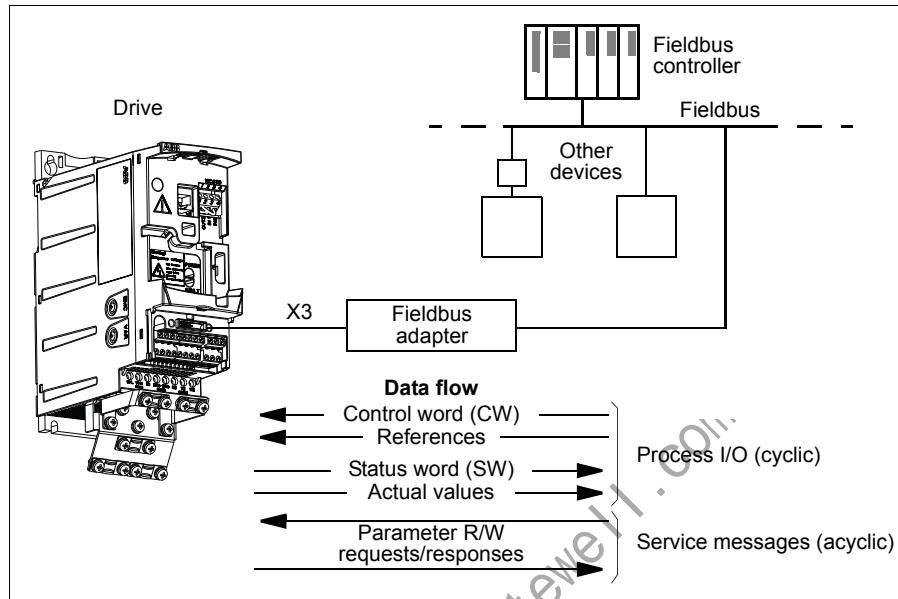
The drive can be set to receive all of its control information through the fieldbus interface, or the control can be distributed between the fieldbus interface and other available sources, eg, digital and analog inputs.
