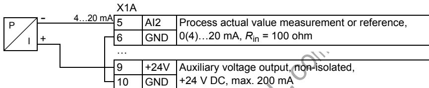
**Note:** The sensor is supplied through its current output and the drive feeds the supply voltage (+24 V). Thus the output signal must be 4...20 mA, not 0...20 mA.
