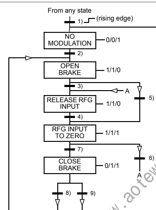
RFG = Ramp function generator in the speed control loop (reference handling).
