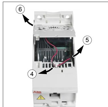
7. Install the new fan holder including the fan in reverse order.
