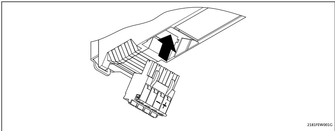
[5-7] Communication via the diagnostic interface (only for Servo Drives 9400)
