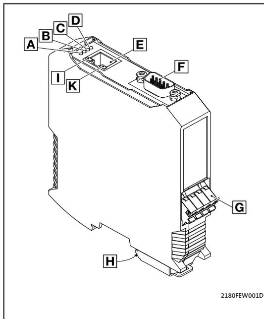
A ... D [LED status displays for the communication module and for CAN communication \(49\)](#)
