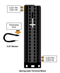
The thermistor end of the CJC sensor must be installed in the CJC1 IN+ or CJC2 IN+ terminal for accurate temperature measurements. The gold pin end of the CJC sensor must be installed in the CJC1 IN- or the CJC2 IN- terminal.
