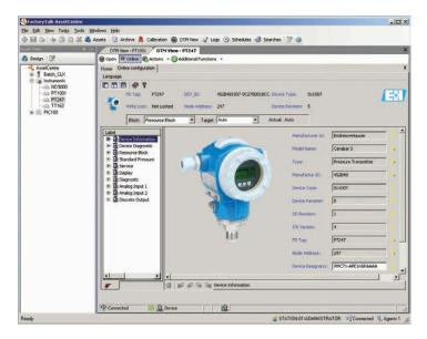
FactoryTalk AssetCentre Process Device Configuration is enabled by FDT Technology. FDT Technology standardizes the communication interface between field devices and host systems to reduce integration efforts.
