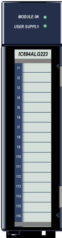
The PACSystems\* RX3i/Series 90\* 16-Channel Analog Current Input module provides 16 single-ended input channels. Each input can be configured using the configuration software for any of three input ranges:
