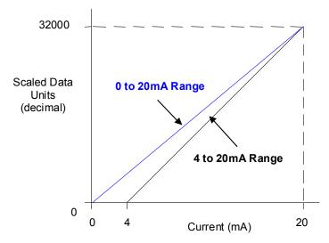
If the current source is reversed into the input or is less than the low end of the current range, the module provides an input data word corresponding to the low end of the current range (0000H in PLC memory). If an input is greater than 20 mA, the module provides an input data value at full scale (7FF8H in PLC memory).
