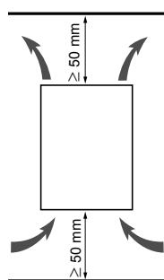
Install the unit vertically, at  $\pm 10^\circ$ .
