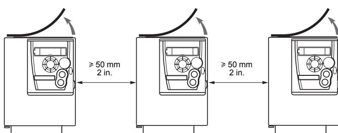
Free space  $\geq 50$  mm (2 in.) on each side. Vent cover should be removed for operation at surrounding air temperature above  $50^\circ\text{C}$  ( $122^\circ\text{F}$ ). The degree of protection becomes IP20
