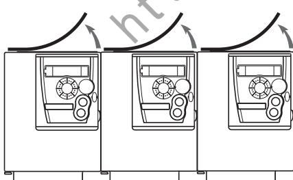
Drives mounted side-by-side, vent cover should be removed (the degree of protection becomes IP20).
