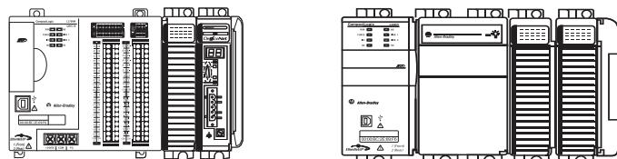
The modules mechanically lock together with a tongue-and-groove design and have an integrated communication bus that is connected from module to module by a moveable bus connector.
