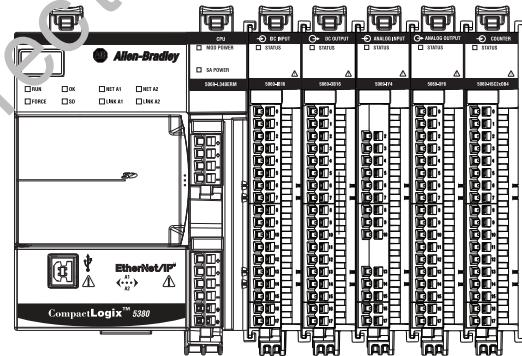
The COMPACT 5000 I/O modules are installed to the right of a CompactLogix 5380 controller and require a separately sold removable terminal block (RTB) to connect field-side wiring.
