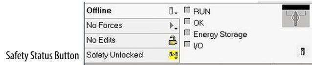
The application tray also displays the following icons to indicate the safety controller's safety-lock status.
