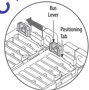
**IMPORTANT** You must install an end cap onto the right side of the Compact GuardLogix 5370 controller system either at the end of the controller or at the end of any local expansion modules that can be installed onto the controller.
