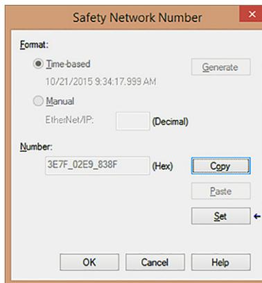
5. Verify that the Network Status (NS) status indicator is alternating red/green on the correct device before clicking Yes on the confirmation dialog box to set the SNN and accept the replacement device.
