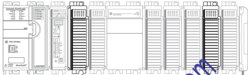
1769-HSC High-speed Counter Modules Installed in a 1769-L36ERMS Control System Meeting the Power Supply Distance Rating Requirements of the High-speed Counter Module
