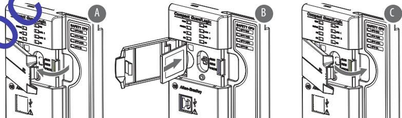
3. Insert the SD card into the SD card slot.
