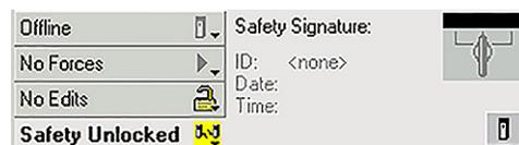
The Safety Status button itself indicates whether the controller is safety-locked or -unlocked, or faulted. It also displays an icon that shows the safety status.
